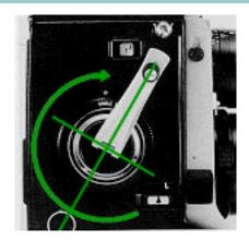
5. Turn the film advance crank clockwise until it stops. The figure 1 appears on the exposure counter at the position where the crank stops diagonally upward, and the shutter is automatically set. Now the camera is ready for the first exposure.
